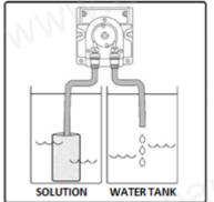
Connect the pump to the timer (or Power Socket 240V AC) The pump will discharge 0,08 cL every 2 seconds.
